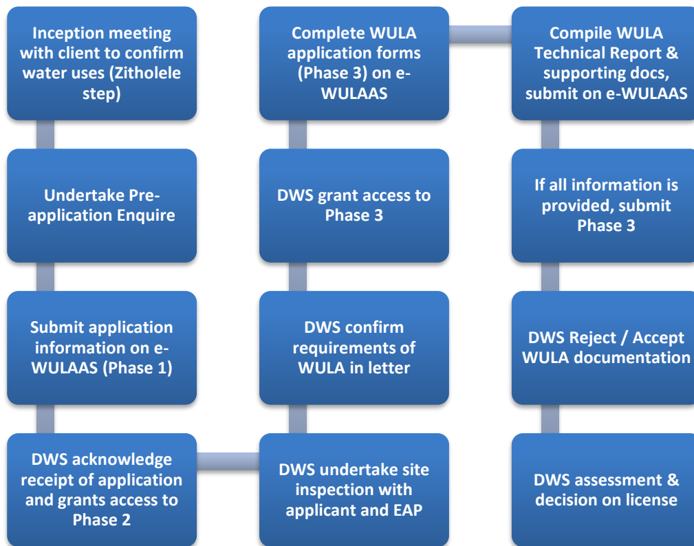
Figure 3: Process Flow Diagram for the steps required in a Water Use License Application
