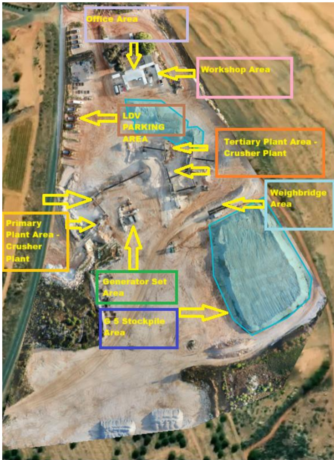
Figure 2-2: The Crusher Plant Layout
